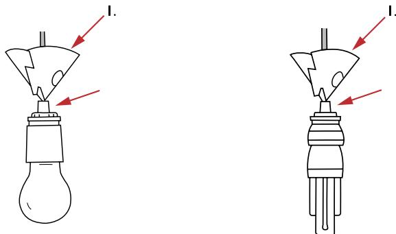
"Snap" the first hanging element around the cable with the point downwards. **IMPORTANT!** There must be a gap between the bulb socket and the hanging element, so the accompanying spacer **MUST** be fitted to the cable as shown in the drawing.
