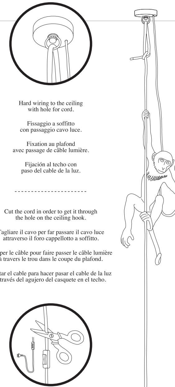
Hard wiring to the ceiling
