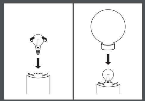
Place a recommended light bulb in the E27 socket
