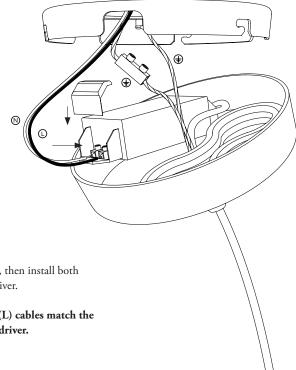
${\bf 5.}\ \ \, {\rm To}$  install the cables, remove the green cap, then install both cables, natural (N) and live (L) into the driver.
