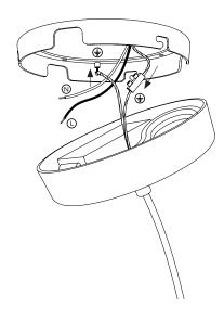
**4.** Connect the earth cable with the loop to the ceiling frame, and the earth cable with the terminal to the earth cable coming out of the ceiling.
