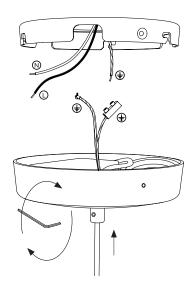
3. Use two fingers to adjust the length of the cord by pushing up or downwards. Roll up the excess cord and place it inside the canopy.
