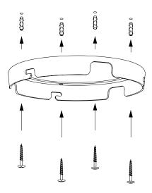
2. Drill holes. Make sure to use plugs and screws appropriate for the ceiling material. Mount the ceiling fitting.
