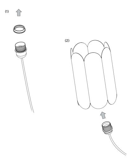
Insert the bulb holder through the central hole in the base plate and clamp it in place by screwing the ring back onto the bulb holder. Take care to fasten the ring securely, especially if you are using the shade with the pendant cord set.
