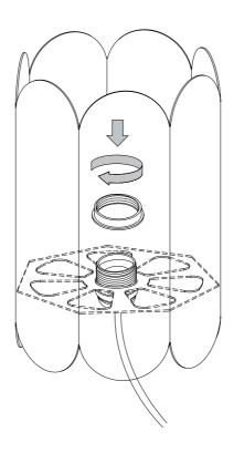
Screw an LED light bulb into the bulb holder.
