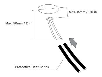
A heat gun can be used to shrink and fix this protective insulation in place, as shown below.
