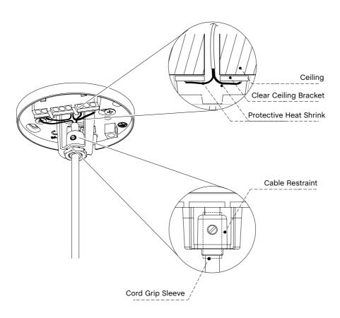
If utilising the mouse hole cable exit, please note the internal cable restraint and integrated cable clamp. The cable clamp tab can be removed and cut to length to suit the cable thickness used, if this is larger than what is already provided.
