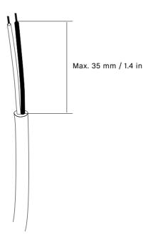
There is a 5 mm / 0.2 in wire strip guide provided on the internal transparent cover, as shown below. Strip 5 mm / 0.2 in of exposed wire carefully, ensuring both layers of insulation are intact and not damaged.
