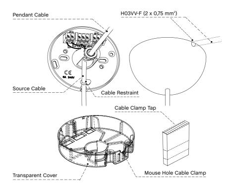
Replace the protective transparent cover over the terminal and clear ceiling bracket, screwing it in place with the three fixings provided. This will isolate the internal electrics during use. Replace the outer magnetic ceiling cap over the assembly, ensuring the mouse hole exits are lined with the bracket and cap if you intend to utilise this feature.
