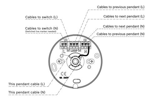
Check to ensure that the protective heat shrink, the cable restraints and cord grip sleeve are still in place after fitting all the wires. Check that all of the Live, Neutral and Ground connections are securely connected before switching the power back on at the mains. Ensure there are no loose cables or exposed bare wires and that the clear ceiling bracket is securely fixed to the ceiling.
