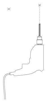
Trim the cable to the desired length, leaving 35 mm / 1.4 in of basic single insulation exposed for wiring.
