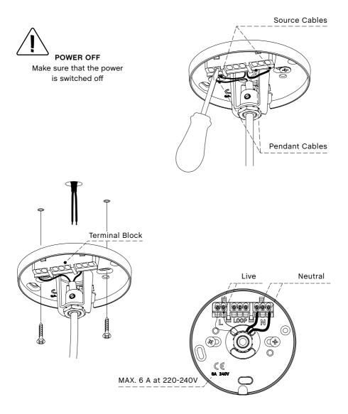
The terminal blocks of the clear ceiling bracket are integrated into a junction box with a loop-in feature. This can be utilised in a number of different ways to optimise the wiring of electrical fittings used in your environment, either for single light fixtures and switches, multiple light fixtures to a single switch, or even lamps and ceiling fans connected to a single switch.
