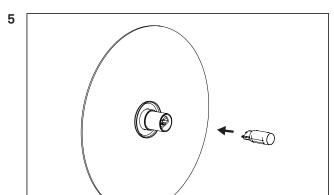
Place a G9 light bulb in the socket. The bulb is NOT included.
