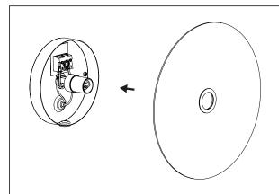
Carefully place the cover plate over the socket.
