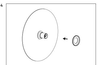
Place the small metal plate over the socket.
