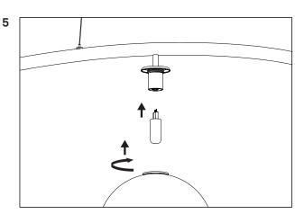
Place a G9 light bulb in the socket. The bulb is NOT included.
