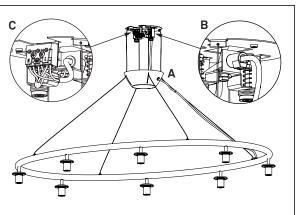
Push the lamp cable through the cover plate (A) and strain relief on the mounting bracket (B). Connect the cable-ends to the cable terminal (C).
