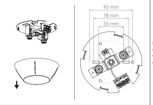
Pull cover plate away from mounting bracket. It is attached with strong magnets and might require some force. 4
