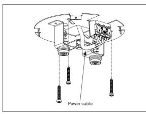
Attach the mounting bracket to the ceiling.
