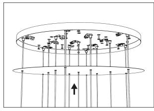
Attach the cover plate to the ceiling plate by carefully sliding it up and let the magnets fixate the cover plate to the ceiling plate.
