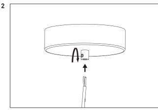
Lead the fabric cable in through the cable relief at the bottom of the ceiling plate. Adjust the cable to the desired length.
