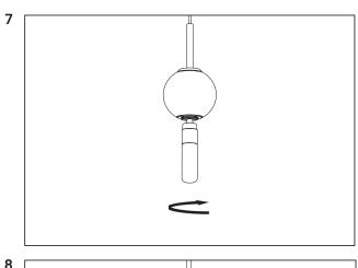
Screw the light bulb into the socket.
