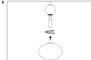
Take the glass globe and carefully place it over the light bulb and socket.
