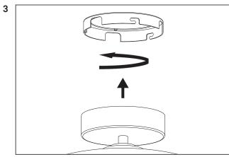
Attach the lamp to the top plate by turning the lamp.
