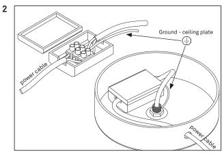
Install the power cable by leading it through either the top or the side of the ceiling plate into the cable connector.
