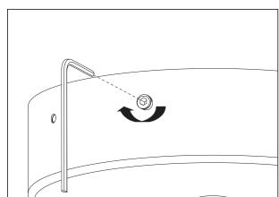
Fixate with the socket screw. Install the socket screw with the Allen key provided.
