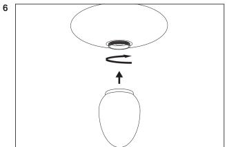
Take the lower glass and carefully place it over the light bulb and socket.
