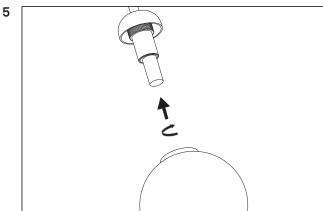
Carefully place the glass globe over the light bulb. Turn clockwise to attach the glass globe.
