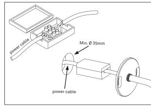
Connect the wire-ends to the cable connector inside the connector box. Match the brown wire with "L" the blue wire with "N" and the green/yellow wire with the grounding symbol.
