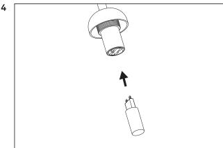
Place a G9 light bulb in the socket. The bulb is NOT
