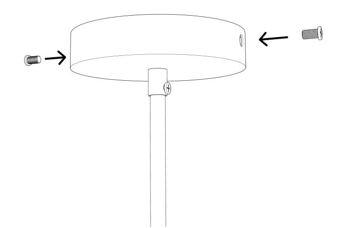
**Step 4** Place the canopy cup onto the metal bracket and secure it in the right position with the including screws.
