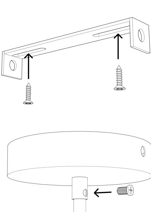
Step 1 Ensure power supply is turned off and remove any existing lamp fitting. Mount the metal bracket (B) securely in the ceiling with screws and wall plugs, appropriate for the ceiling of installation.
