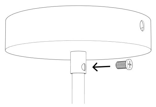
**Step 2** To determine the right suspension height for the lamp, pass the electrical cord through the strain relief of the canopy (B). When you have the desired suspension height of the lamp, tighten the plastic screw of the strain relief.
