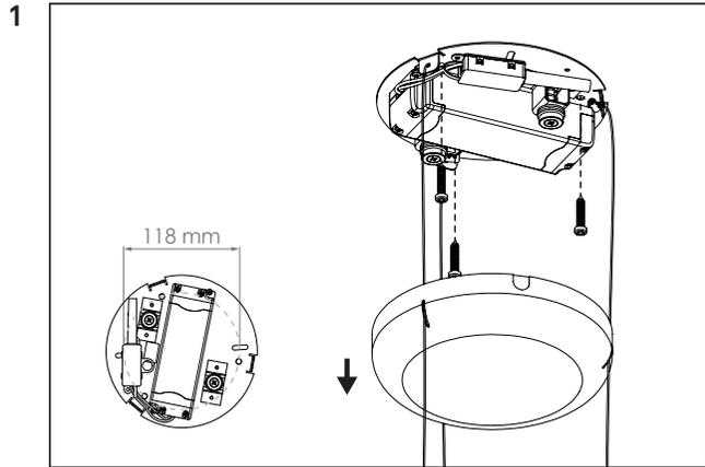
Remove the cover on the canopy. Magnets hold the cover in place.
