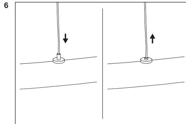
Use the wire locks on the ring to adjust the lamp to its final position. It is recommended to use a spirit level.
