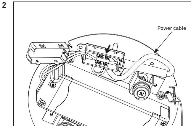
Lead the power cable through the hole in the mounting bracket and into the connector box.
