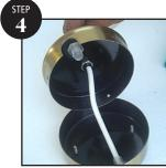
Unscrew this plate from the screws shown with the help of a screwdriver.
